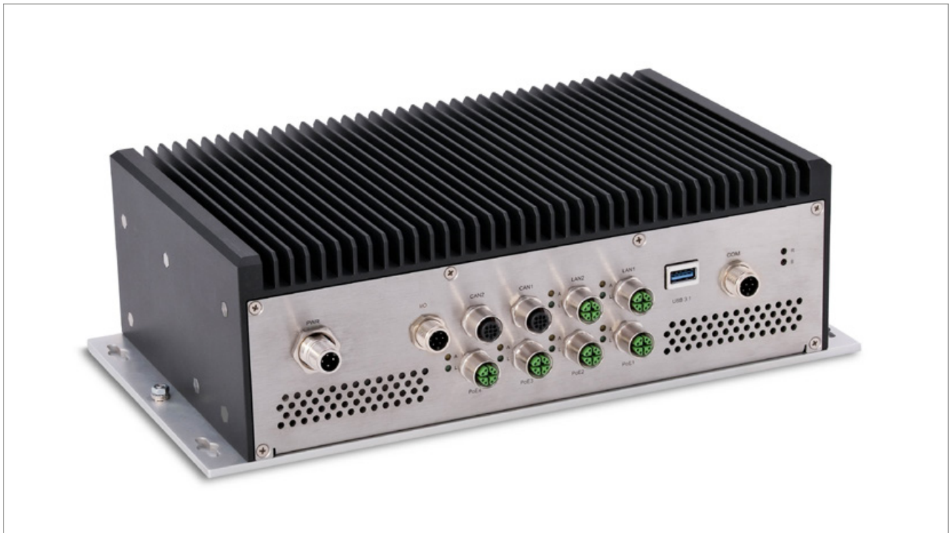
AI railway computer RML A4AGX – powered by NVIDIA Jetson AGX Orin KI Railway Computer RML A4AGX – basierend auf NVIDIAs Jetson AGX Orin SoM
