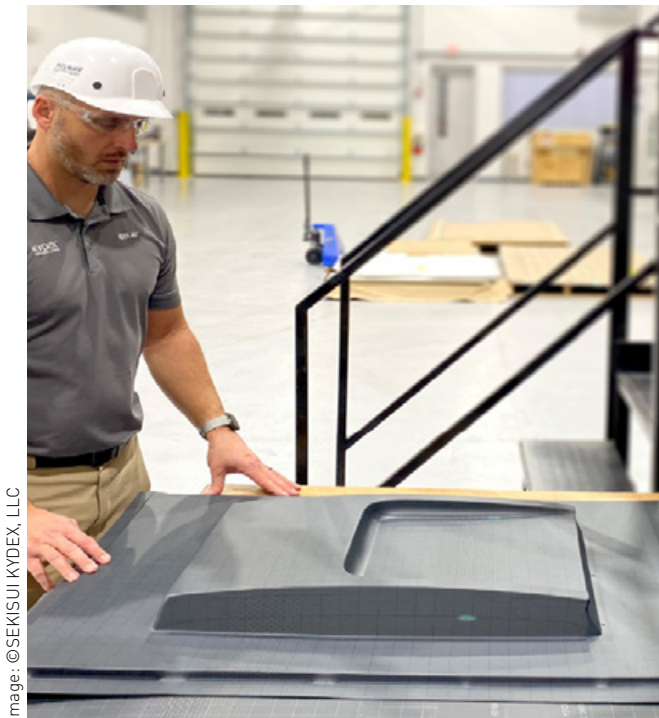
Thermoforming KYDEX® thermoplastics Thermoformung von KYDEX® Thermoplastics
