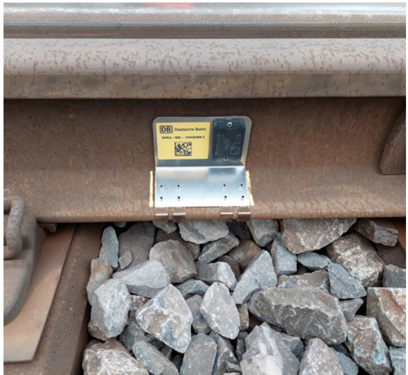
Rail clamp on the track bed with new clamp mechanism including barbs Schienenklemme am Gleißbett mit neuem Klammermechanismus inklusive Widerhaken
