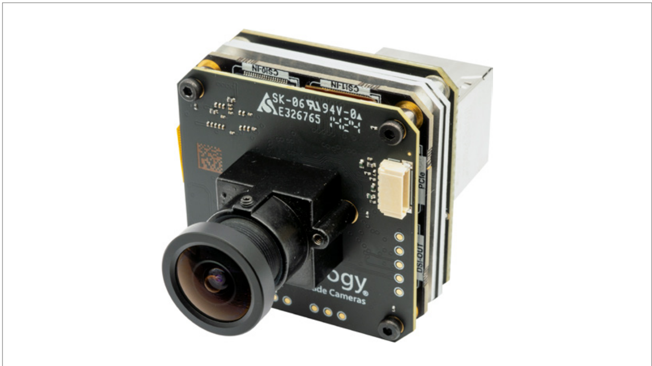
SCAiLX Edge AI camera platform SCAiLX Edge-AI Kameraplattform
