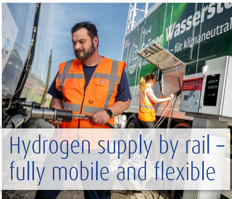
Rapid refuelling with a mobile filling station and hydrogen storage trailer
