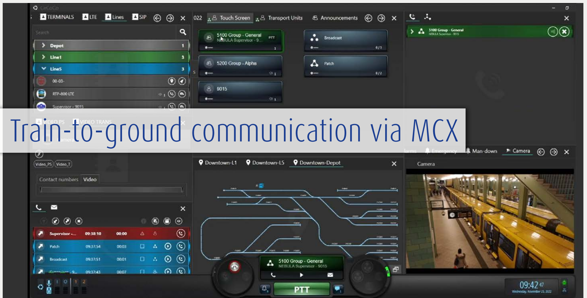
NG CeCoCo integrates MCx communication in the control room with applications such as video
