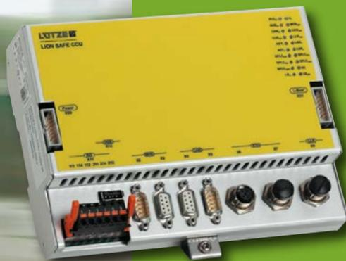
The new LION Safe CCU expands the LION product family with a powerful control unit that is SIL2-capable. With the L-Bus<sup>2</sup>, the controller can be easily adapted to any application. Various safe and non-safe IO modules are available for this purpose.
