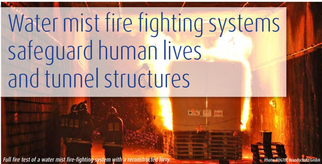
Full fire test of a water mist fire-fighting system with a reconstructed lorry.
