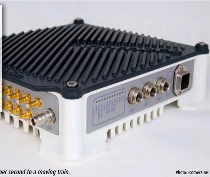
The Icomera X5 router delivers over 1 gigabit of data per second to a moving train.
