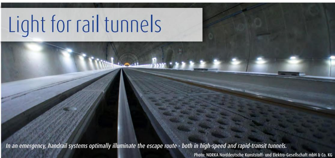
In an emergency, handrail systems optimally illuminate the escape route - both in high-speed and rapid-transit tunnels.
