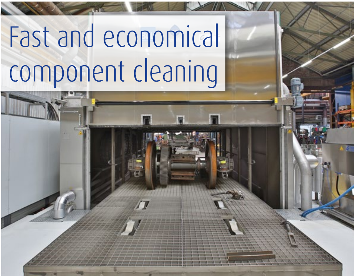
Efficient cleaning of wheelsets and bogies using the Pacific cleaning system.
