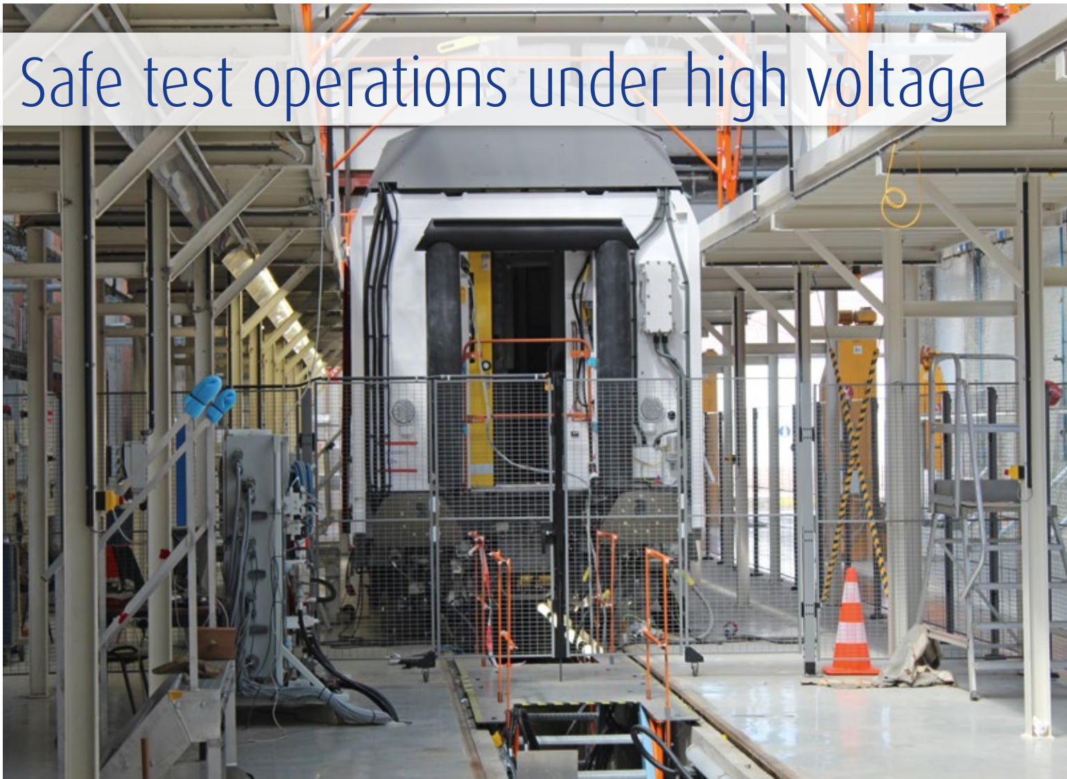
Safety first: In a test cage the rail vehicles undergo dozens of functional and electric tests.
